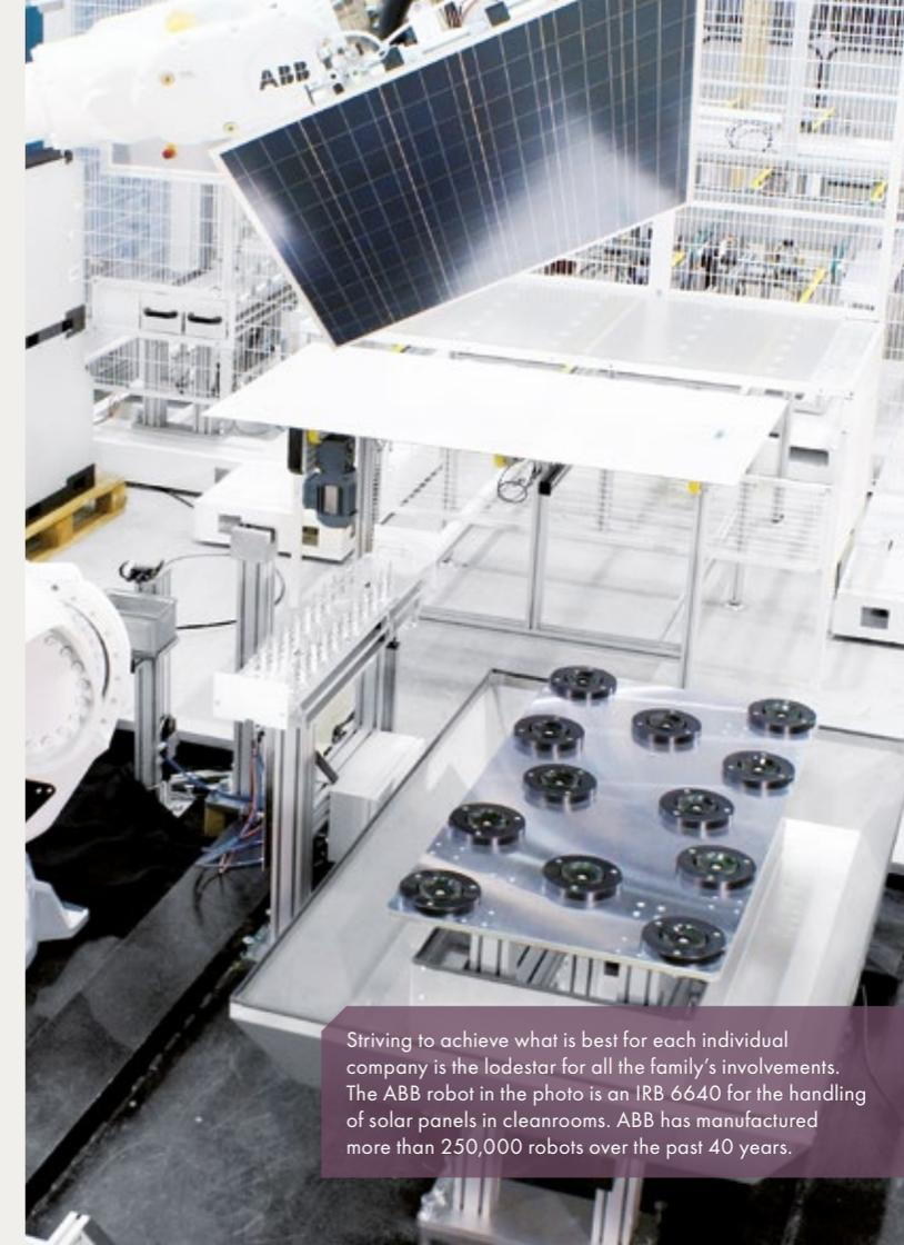
Striving to achieve what is best for each individual company is the lodestar for all the family’s involvements. The ABB robot in the photo is an IRB 6640 for the handling of solar panels in cleanrooms. ABB has manufactured more than 250,000 robots over the past 40 years.
